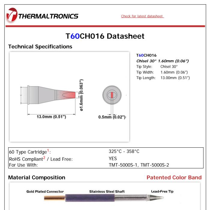
Chromium/Nickel Iron Plating Copper Core Solder
