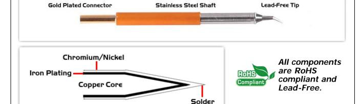
Thermaltronics tip cartridges will typically idle within a temperature range of +/-1.1°C. However, there is variation in idle temperature across tip geometries within an individual temperature series. Thermaltronics offers a wide variety of tip geometries from 0.25mm fine point tip to 5mm chisel. The length and geometry of a tip will have an influence on the tip idle temperature. To accurately measure idle temperature it will depend greatly on the measurement method,
